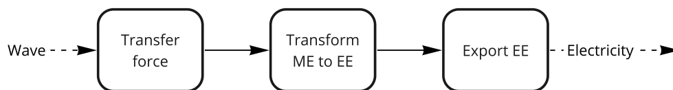
Fig. 2: Simple Functional Decomposition of Submerged WEC
